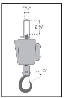
Figure 3. Scale side view measurements.
